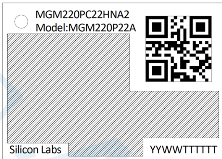
Figure 8.3. MGM220P Top Marking
