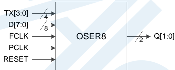
Figure 3-25 I/O Logic in OSER8 Mode
