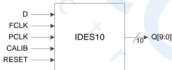
Figure 3-26 I/O Logic in IDES10 Mode
