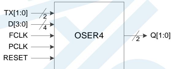
Figure 3-21 I/O Logic in OSER4 Mode
