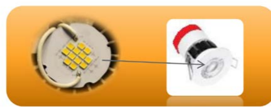
LED module in a "containing product" / luminaire
