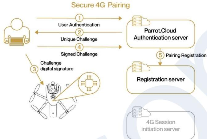
Then, Parrot servers register the association between the user and the drone. When Wi-Fi connection between the user and the drone is lost, ANAFI Ai automatically connects in 4G. ANAFI Ai does a strong authentication on Parrot servers, using its private key stored on the Secure Element. Parrot servers look for the associated users and enables pairing between ANAFI Ai and the Skycontroller 4.
