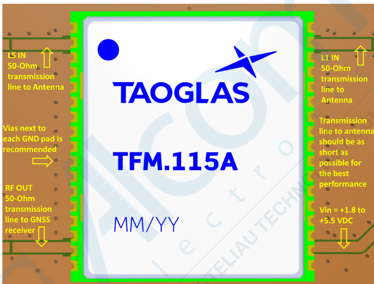
TFM.115A module mounted on a PCB, showing transmission lines and integration notes.
