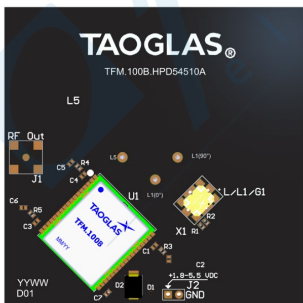
Bottom side (TFM.100B placement including HC125A )
