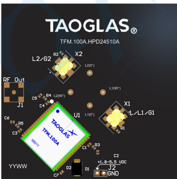
Top Side ( HP24510A placement on 70x70mm PCB)
