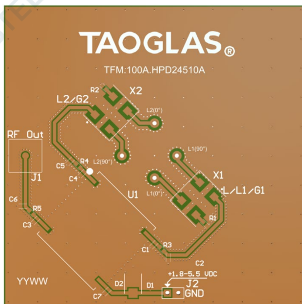
Top Side ( HP24510A placement on 70x70mm PCB)
