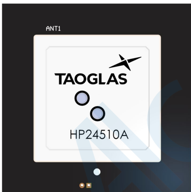
Top Side ( HP24510A placement on 70x70mm PCB)
