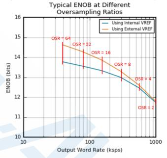
Figure 4.14. Typical ENOB vs. Oversampling Ratio
