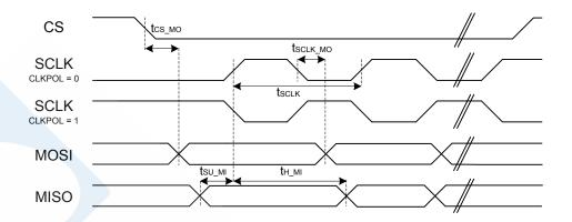
Figure 4.7. SPI Main Timing
