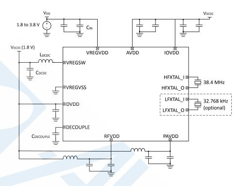
Figure 5.2. Typical Application Circuit: Buck DCDC Configuration with PAVDD, RFVDD, AVDD, and IOVDD from DCDC output (EFR32xG27C1x)
