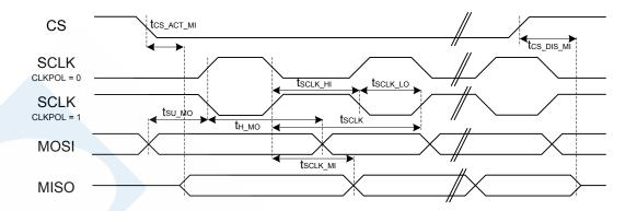
Figure 4.6. SPI Secondary Timing
