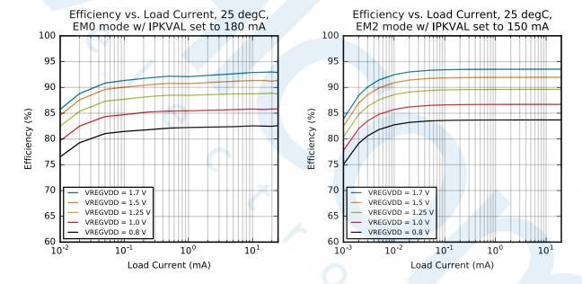
Figure 4.13. Boost DC-DC Efficiency
