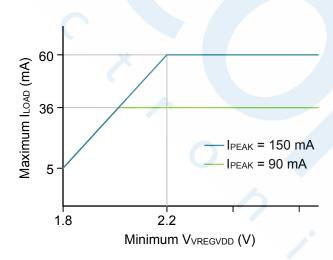
Figure 4.2. Transient maximum load current vs. Minimum input voltage
