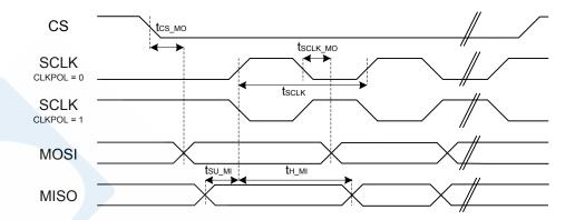
Figure 4.4. SPI Main Timing (SMSDELAY = 0)
