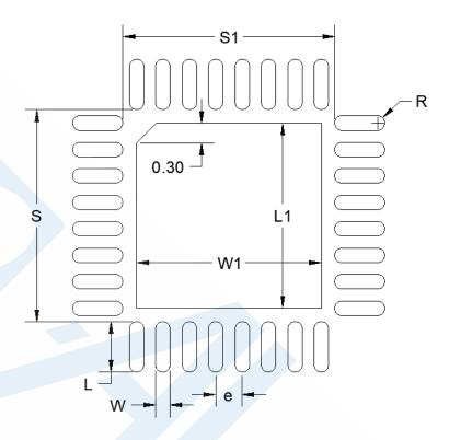
Figure 7.2. QFN32 PCB Land Pattern Drawing
