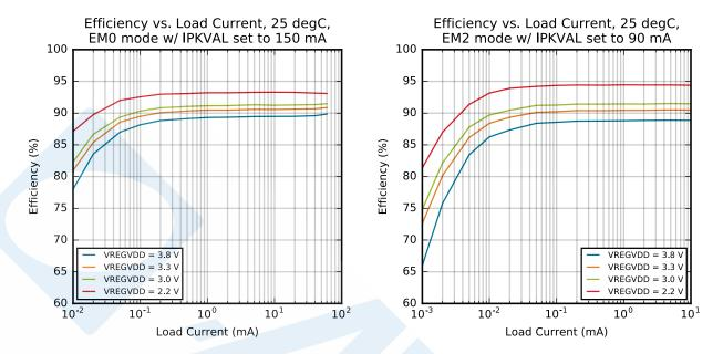
Figure 4.12. Buck DC-DC Efficiency
