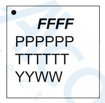
Figure 8.3. QFN40 Package Marking
