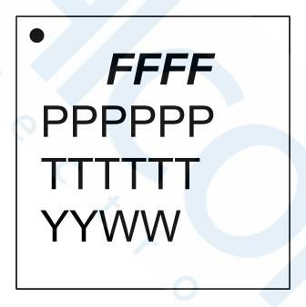
Figure 7.3. QFN32 Package Marking
