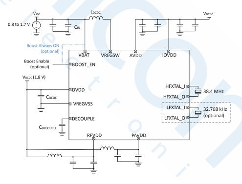
Figure 5.3. Typical Application Circuit: Boost DCDC Configuration with PAVDD, RFVDD, AVDD, and IOVDD from DCDC output (EFR32xG27C2x)
