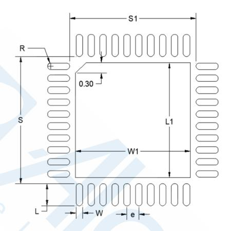
Figure 8.2. QFN40 PCB Land Pattern Drawing
