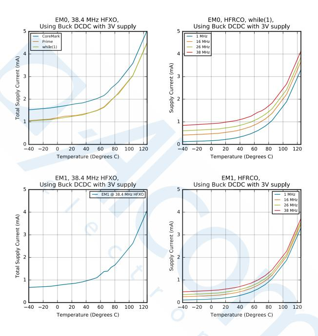
Figure 4.9. EM0 and EM1 Typical Supply Current vs. Temperature (Buck DCDC)
