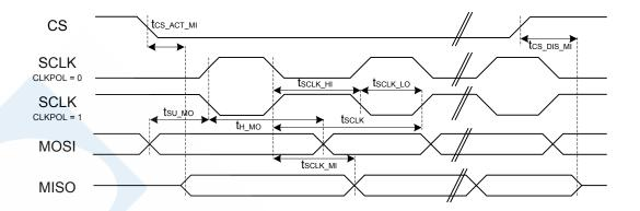
Figure 4.8. SPI Secondary Timing
