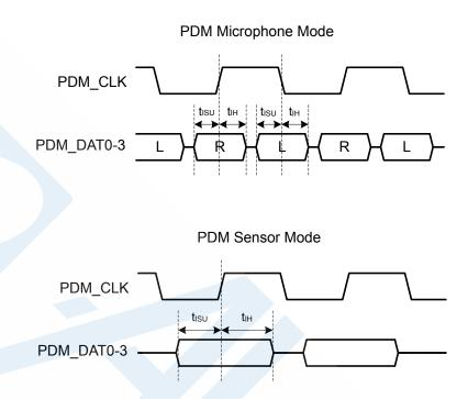
Figure 4.3. PDM Timing Diagrams
