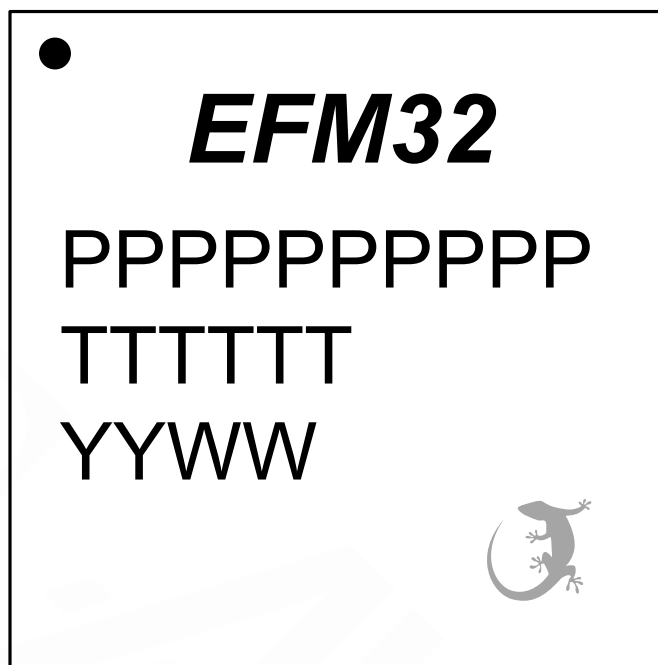
Figure 8.3. QFN40 Package Marking
