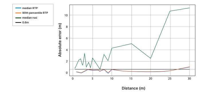
In general, the goal for phase ranging accuracy is less than 60 cm. As shown above, phase range measurements are stable and below the 60 cm error threshold up to 25 m and within one meter accuracy up to 30 m. With RSSI, it's unlikely to achieve sub-meter accuracy even over small distances, plus the error rate will only increase with distance, reaching more than 10m error above distances of 25m.
