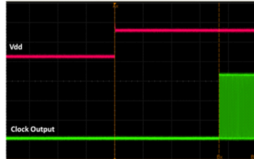
Figure 14. Startup Waveform vs. Vdd
