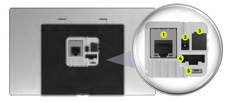
1. RJ-45 3. KNX Bus (2Wire) 5. USB Micro AB (OTG)
