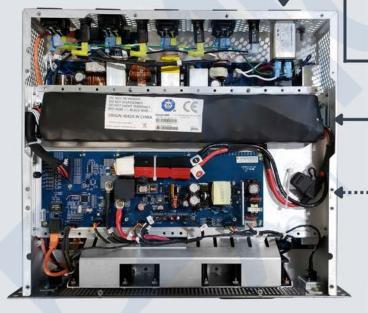
The PowerBridge™ UPS by Astrodyne TDI is a compact, high density, and lightweight solution, perfect to support the digital healthcare industry. It is an all-in-one power solution that includes isolation, LiFePO4 battery, and IEC 60601 certification, in an easy-to-install system.
