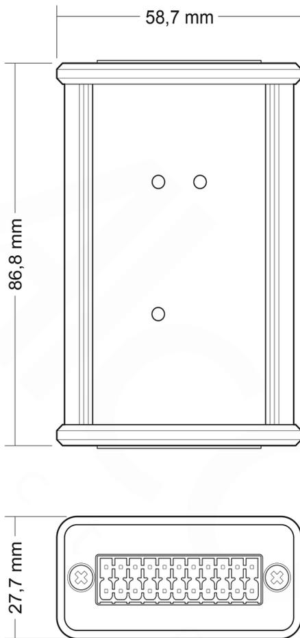
Figure 5: Dimension drawing with top view and side view.
