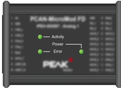
Figure 4: LEDs on the PCAN-MicroMod FD Analog 1
