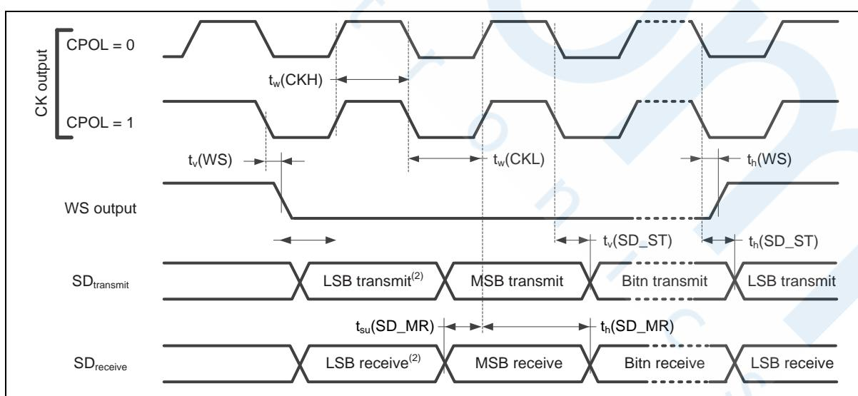
Figure 8.6-5 I<sup>2</sup>S Master Mode Timing Diagram
