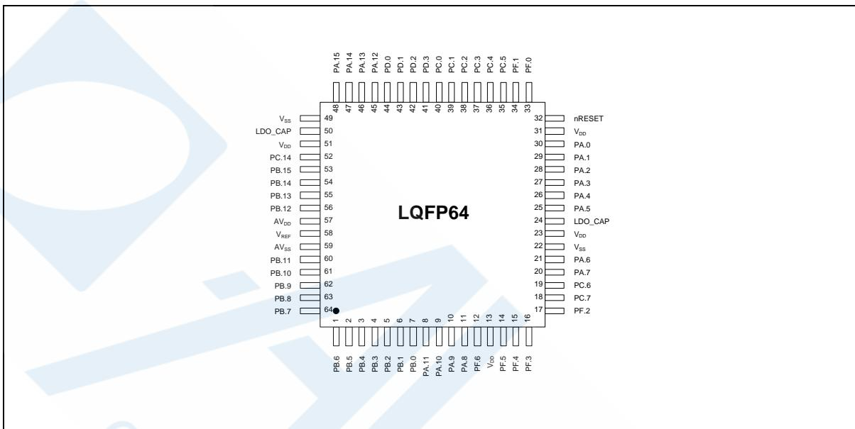
Figure 4.1-2 LQFP-64 Pin Diagram
