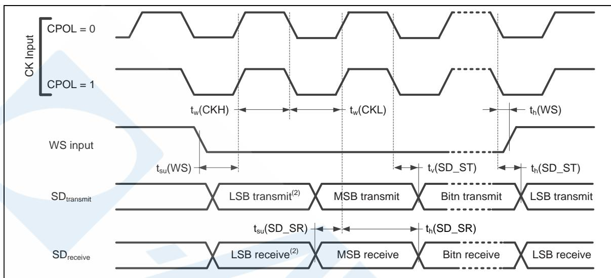
Figure 8.6-4 I<sup>2</sup>S Slave Mode Timing Diagram
