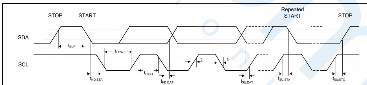
Figure 8.6-7 I<sup>2</sup>C Timing Diagram
