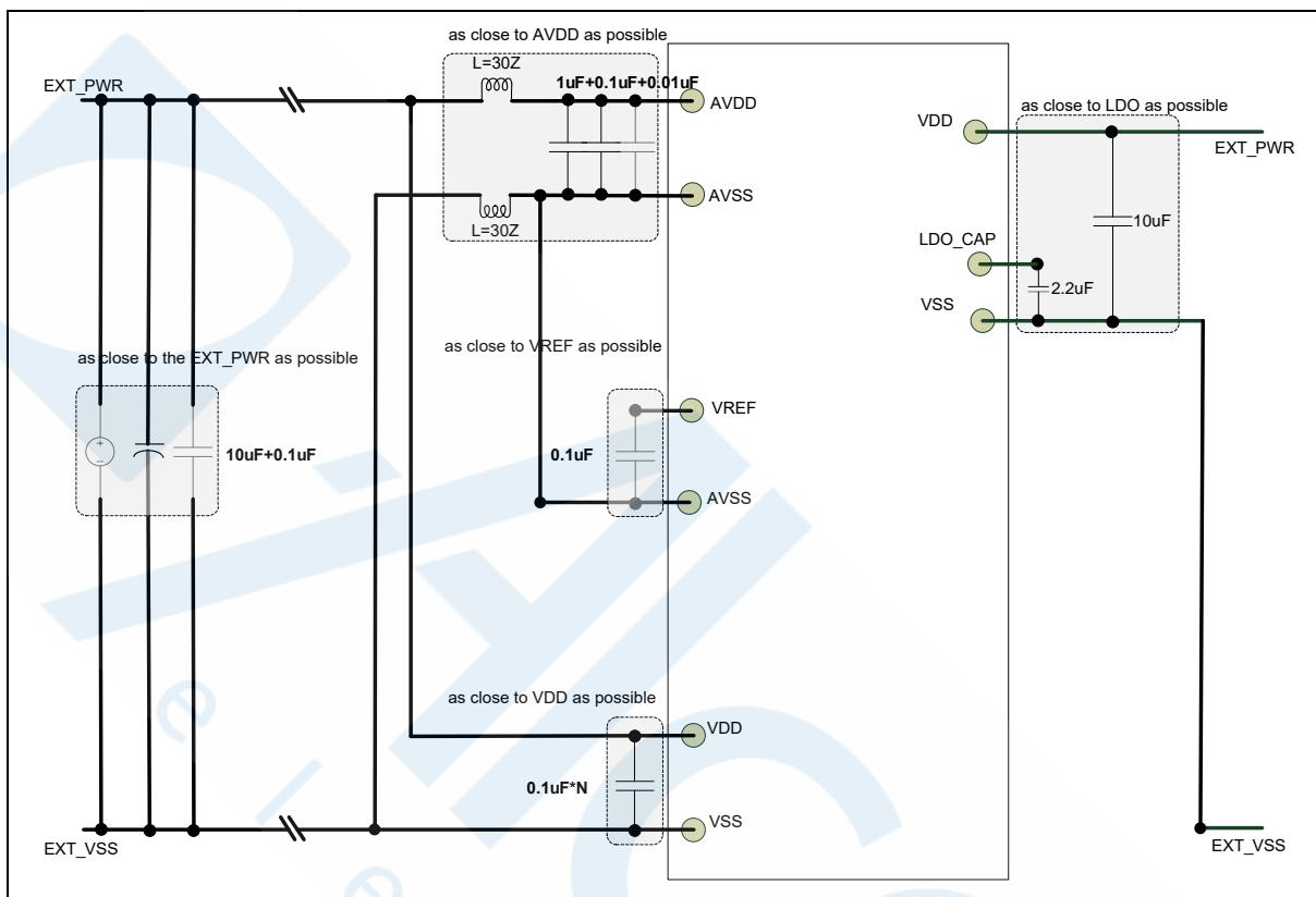
**Note:** Total capacitance of LDO\_CAP pin is 2.2uF.
