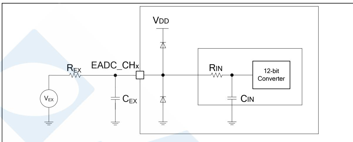
**Note:** Injection current is an important topic of ADC accuracy. Injecting current on any analog input pins should be avoided to protect the conversion being performed on another analog input. It is recommended to add Schottky diodes (pin to ground and pin to power) to analog pins which may potentially inject currents.
