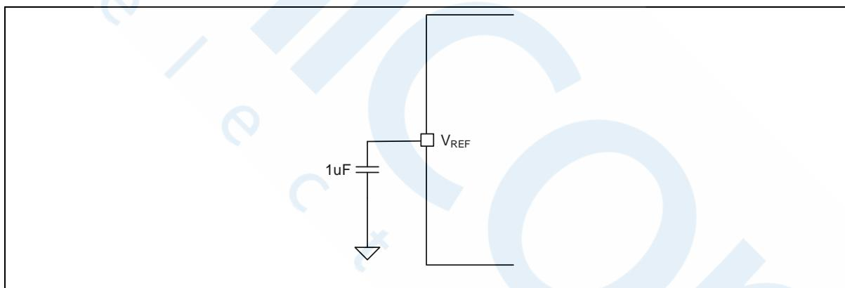
Figure 8.5-2 Typical Connection with Internal Voltage Reference
