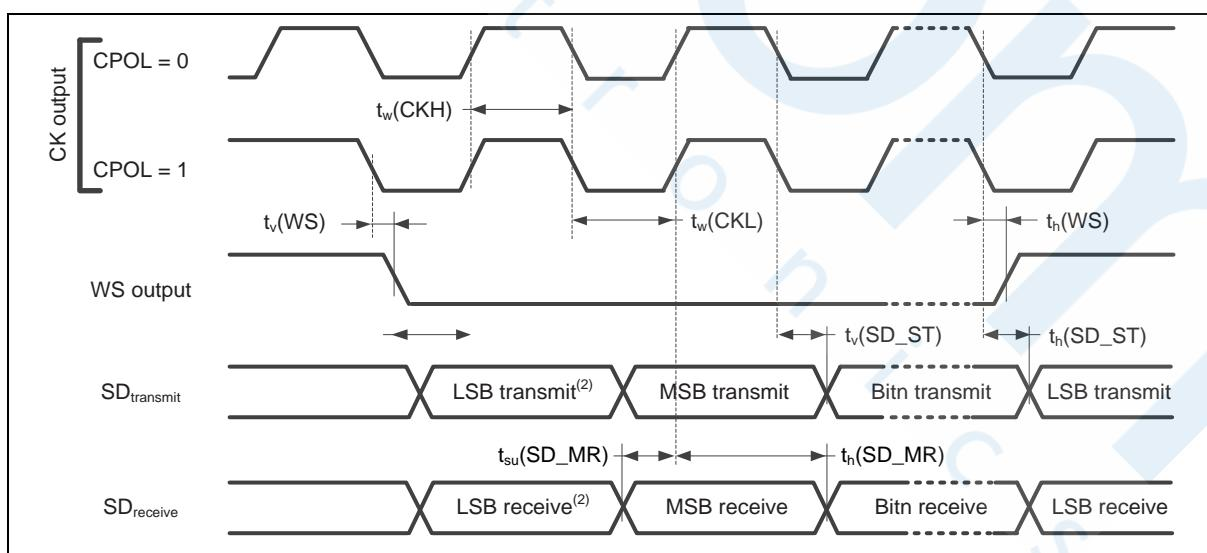
Figure 8.6-3 I<sup>2</sup>S Master Mode Timing Diagram
