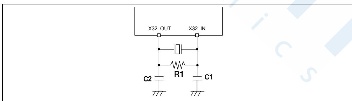
Figure 8.4-2 Typical 32.768 kHz Crystal Application Circuit
