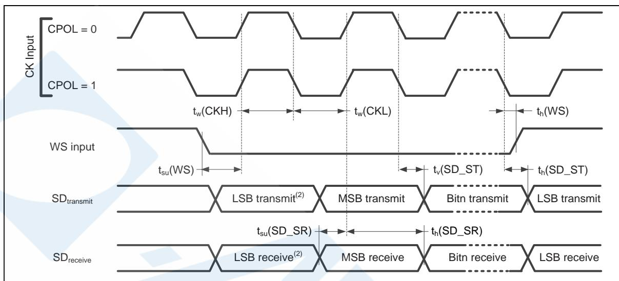
Figure 8.6-6 I<sup>2</sup>S Slave Mode Timing Diagram
