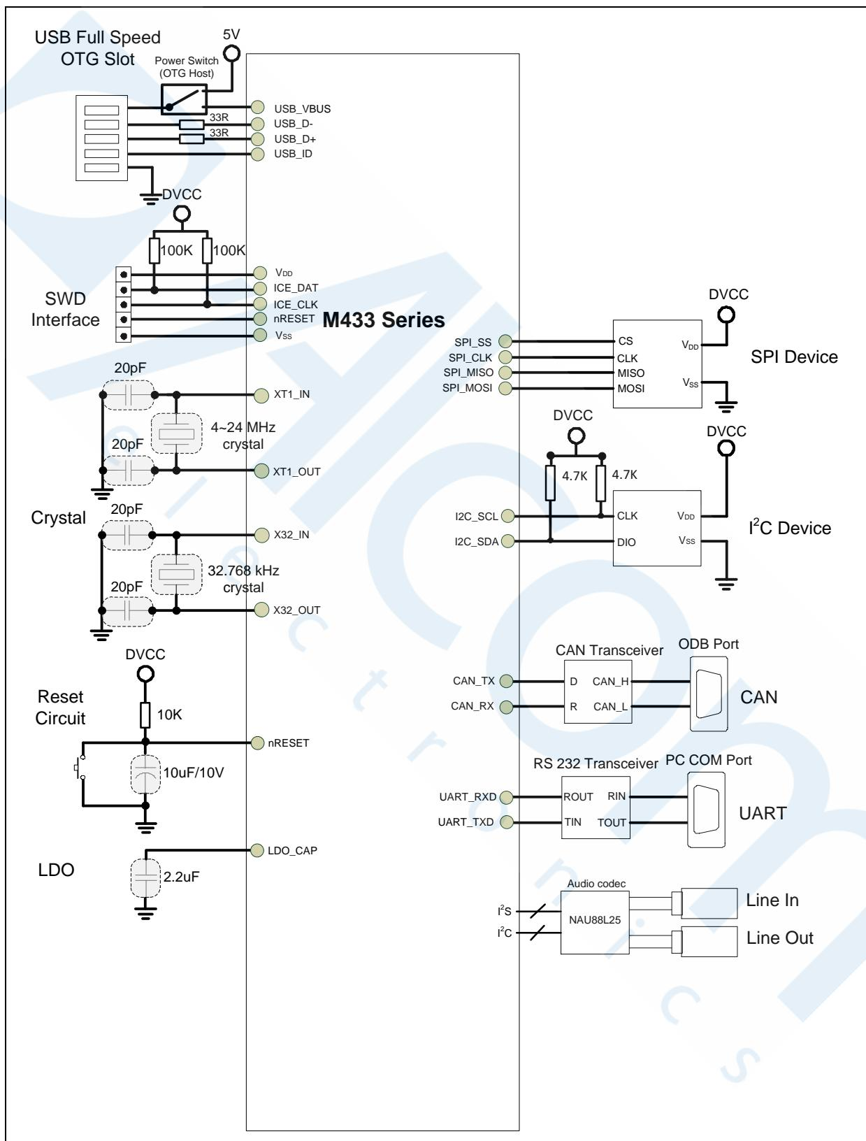
**Note 1:** USB\_ID could be floating using USB without OTG.
