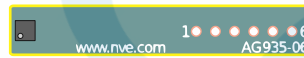
AG035-06: DFN6 connection board for -10E suffix sensors. (1.57" x 0.25" / 40 mm x 6 mm; actual size).
