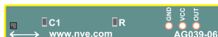
Part Number AG039-06: DFN4 Digital Sensor Board with locations for 0402-size pull-up resistors and bypass capacitors (1.57" x 0.25" / 40 x 6 mm, actual size).
