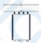
**Notes:** 1) Package contents include DIN Rail clips and associated hardware for mounting devices in the orientation shown above. 2) Clips onto 35mm and 32mm DIN rails.
