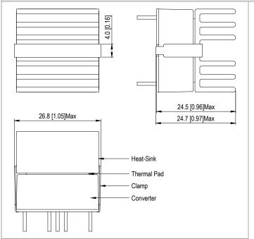
Heatsink Material: Aluminum Finish: Anodic treatment (black) Weight: 6g
