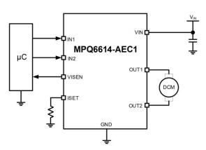
The MPQ6614-AEC1 has a pulse-width modulation (PWM) input interface, which is compatible with industry-standard devices. A brake is applied when stopping the motor. When disabled, the MPQ6614-AEC1 can achieve a low standby circuit current.
