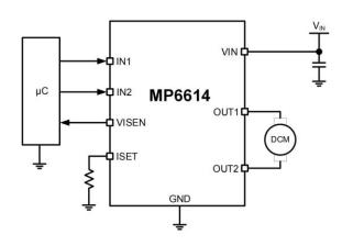
standard devices. A brake is applied to stop the motor, and a very low standby circuit current can be achieved when the device is disabled.
