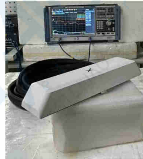
VNA Test Set-up
