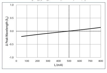
Temperature:  $\Delta \lambda_d = \lambda_d(T_c) - \lambda_d(25^{\circ}C)$ , 20 ms pulse,  $I_f = 500$  mA
