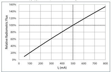
Temperature:  $\varphi_{r}/\varphi_{r}(25^{\circ}\text{C})$ , 20 ms pulse,  $I_{r}$  = 500 mA
