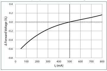
Temperature:  $\Delta V_f = V(T_c) - V(25^{\circ}C)$ , 20 ms pulse,  $I_f = 500$  mA
