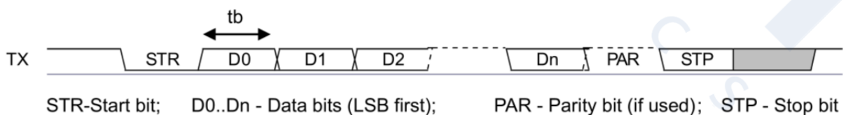
Figure 6-7. UART Data Frame
