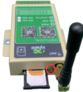
Figure 3-1-5 Installing the SIM card of the InDTU324
