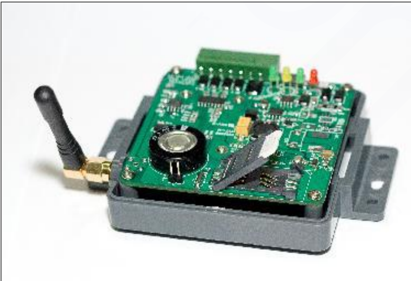
Figure 3-1-2 Installing SIM card into DTU332
