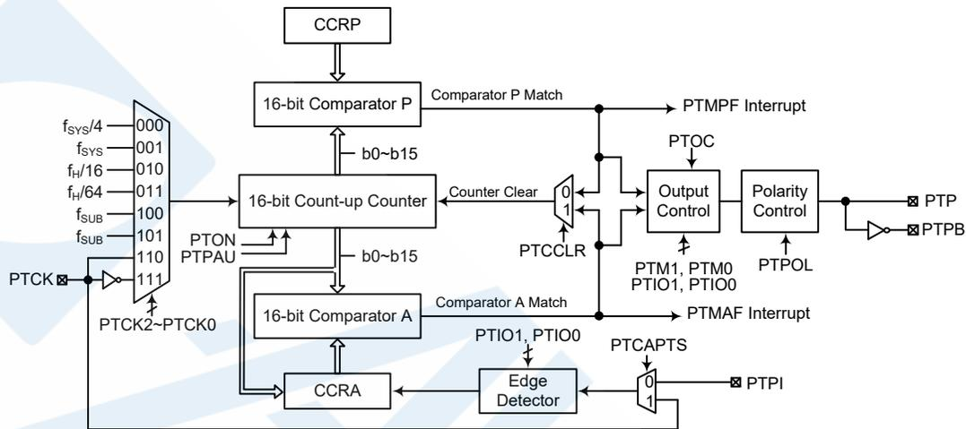
Note: 1. The PTM external pins are pin-shared with other functions, so before using the PTM function, the relevant pin-shared function registers must be set properly to enable the PTM pin function. The PTCK and PTPI pins, if used, must also be set as an input by setting the corresponding bit in the port control register.
