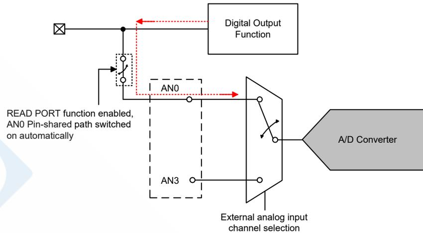
**A/D Channel Input Path Internally Connection**
