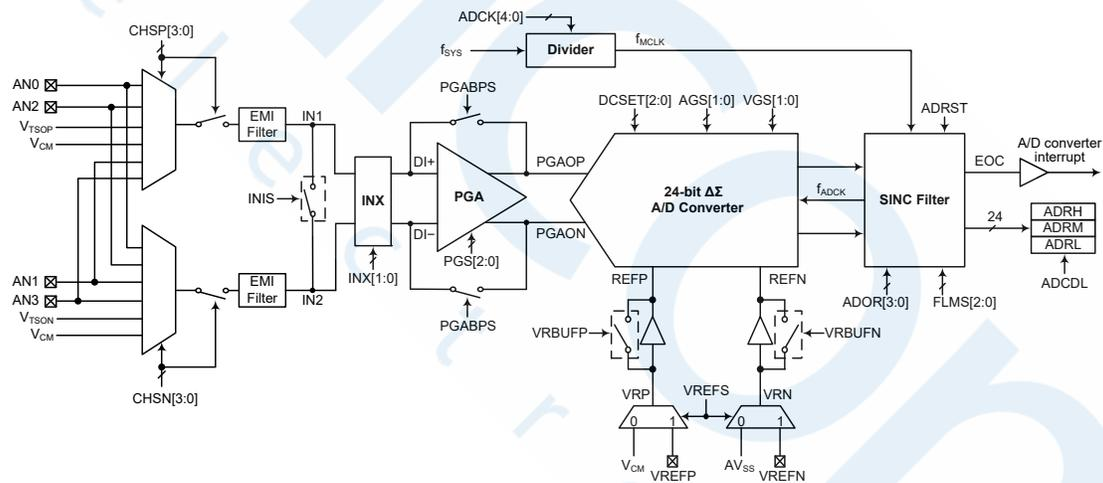
Note: The PGA and A/D converter are power supplied by the  $V_{OREG}$  and  $AV_{SS}$ . The SINC Filter is power supplied by the  $V_{DD}$  and  $V_{SS}$ .
