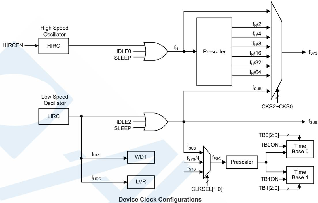
Note: When the system clock source  $f_{SYS}$  is switched to  $f_{SUB}$  from  $f_H$ , the high speed oscillator will stop to conserve the power or continue to oscillate to provide the clock source,  $f_H \sim f_H/64$ , for peripheral circuit to use, which is determined by configuring the corresponding high speed oscillator enable control bit.
