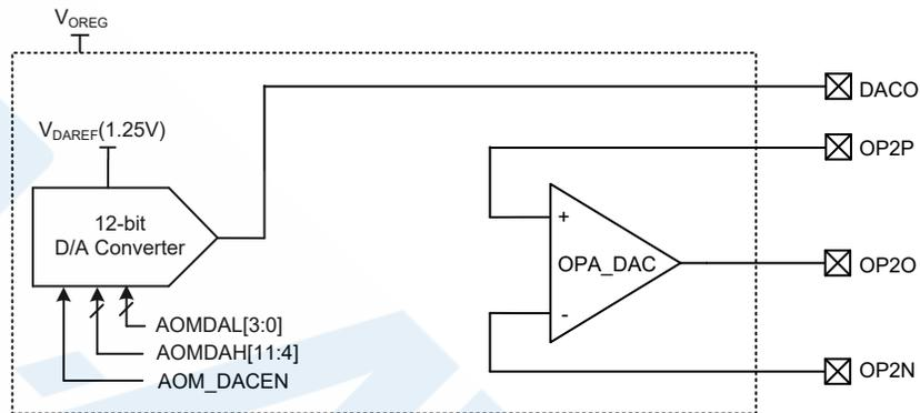
**12-bit D/A converter and OPA Structure**
