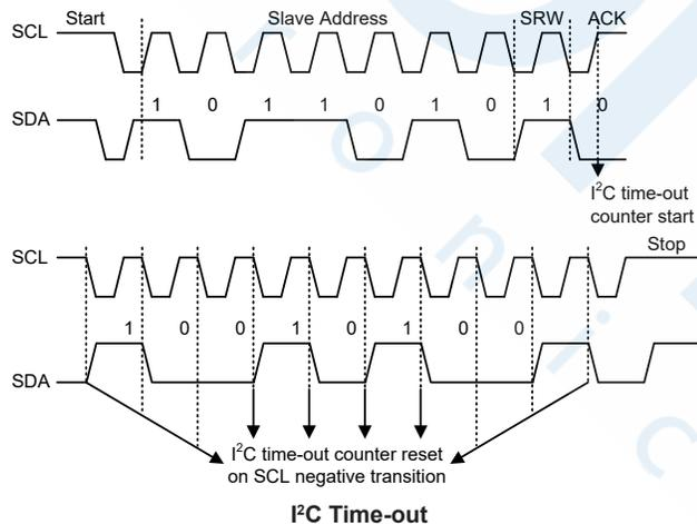
When an I<sup>2</sup>C time-out counter overflow occurs, the counter will stop and the SIMTOEN bit will be cleared to zero and the SIMTOF bit will be set high to indicate that a time-out condition has occurred. The time-out condition will also generate an interrupt which uses the USIM interrupt vector. When an I<sup>2</sup>C time-out occurs, the I<sup>2</sup>C internal circuitry will be reset and the registers will be reset into the following condition:
