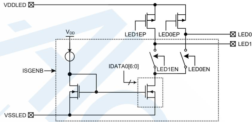
Sink Current Generator Block Diagram
