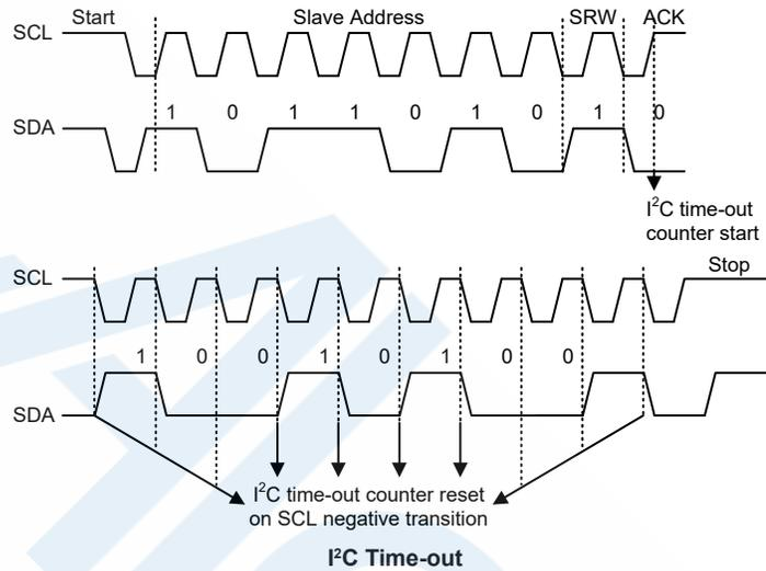
When an I<sup>2</sup>C time-out counter overflow occurs, the counter will stop and the SIMTOEN bit will be cleared to zero and the SIMTOF bit will be set high to indicate that a time-out condition has occurred. The time-out condition will also generate an interrupt which uses the SIM interrupt vector. When an I<sup>2</sup>C time-out occurs, the I<sup>2</sup>C internal circuitry will be reset and the registers will be reset into the following condition:
