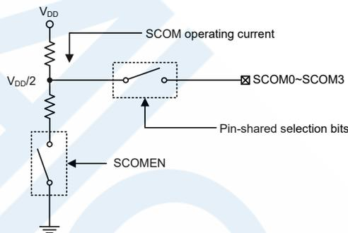
Software Controlled LCD Driver Structure
