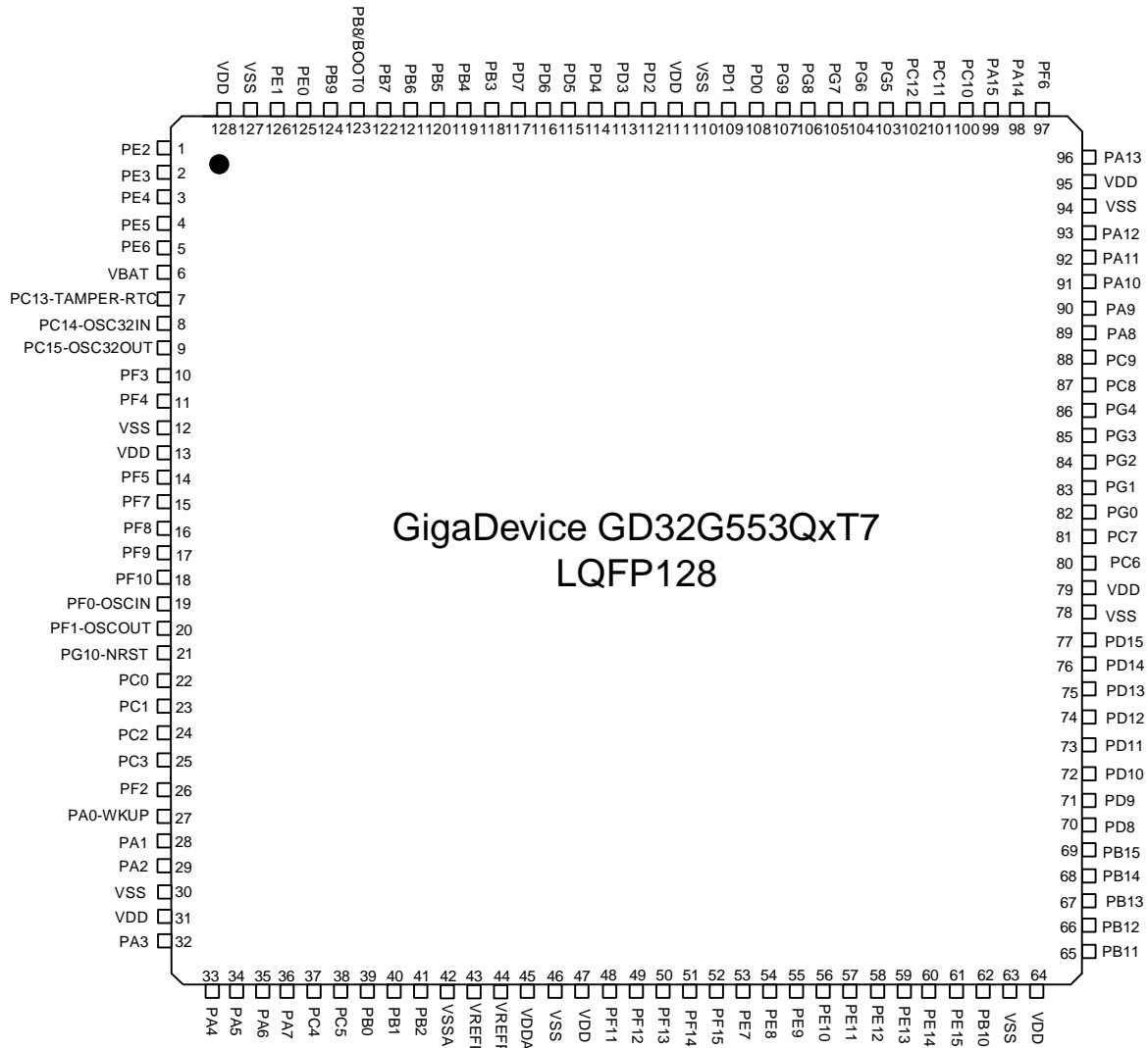
Figure 2-2. GD32G553QxT7 LQFP128 pinouts
