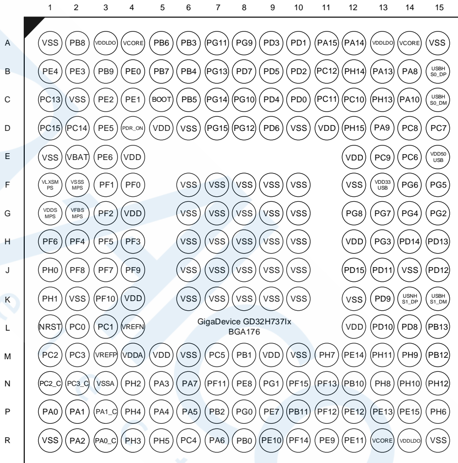
Figure 2-2. GD32H7371x BGA176 pinouts
