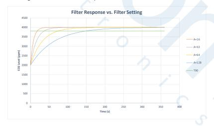
The graph above shows the effect of the filter on response times. Increasing the filter setting increases the measurement output response time.  $T_{90}$  is the time to 90% of reading. The ExplorIR®-W takes 2 readings per second.
