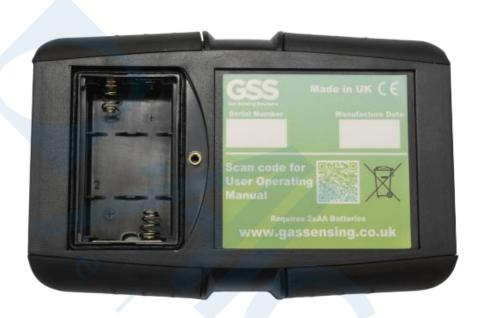
Insert the batteries as per the directions on the battery compartment Replace and screw down the battery cover The unit is now ready for use
