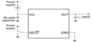
\* Disable current test should be OE = GND. Stand-by current test should be  $\overline{ST} = GND$ .
