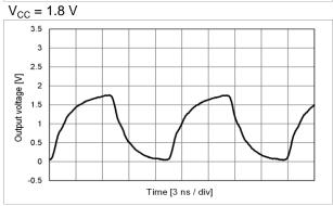
fo = 100 MHz, L\_CMOS = 15 pF, T\_use = +25 °C, Rise/Fall time: A (Default) or C (Fast)
