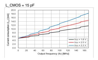
The actual current consumption is the total of the current under the condition of no load and the current to drive the output load (fo x L\_CMOS x V<sub>CC</sub>). To reduce the current consumption, it is effective to use lower frequency, lower supply voltage and lower output load.
