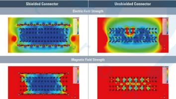
The large-scale shield concept reliably diverts interference currents via the multiple contacting points to both PCBs in the direction of the ground connection.
