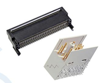
The MicroTCA and AdvancedTCA connectors in press-fit technology enable high data transfer rates. The flat plate press-fitting technique enables efficient press-fitting. The  $\mu$ TCA system uses a straight connector located directly on the backplane, whereas the ATCA system uses the angled AMC connector on the daughter card.
