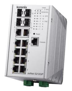
Korenix JetNet 5212GP, the DIN-Rail type industrial Gigabit Managed PoE Switch is designed with eight 10/100/1000TX ports, two Gigabit RJ-45 / SFP combo ports and two Gigabit SFP port. JetNet 5212GP is the first industrial ethernet switch compliance with IEEE 802.3af/at/bt, each ethernet port can max supports 90W for PD, and total budget up to 480W \*Note.
