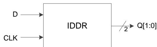
Figure 3-16 I/O Logic in DDR Input Mode
