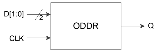
Figure 3-17 I/O Logic in DDR Output Mode
