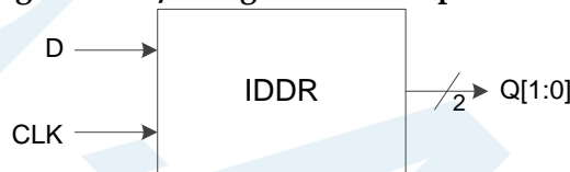
Figure 3-13 I/O Logic in DDR Input Mode
