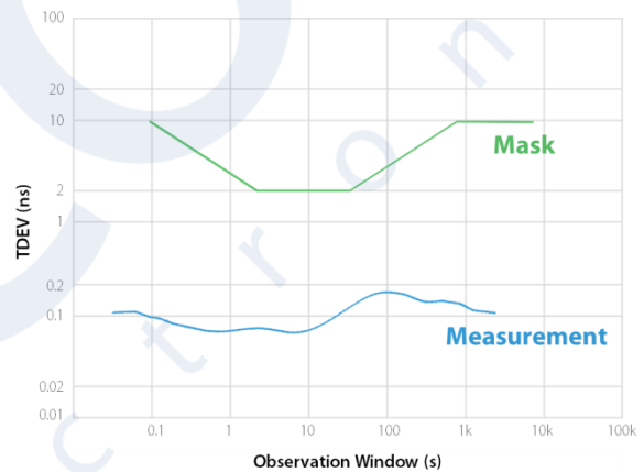
10 MHz G.8262 Option 2 TDEV performance, 0.1 Hz bandwidth
