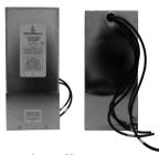
The **059 Series** offers current ratings up to **50 A** @ **60°C**, with 100dB **attenuation from 5 MHz to 10 GHz**. This product line features a compact design and sealed construction with a removable shielded cover for input connections through knockouts. This solution meets IP Class IP65.
