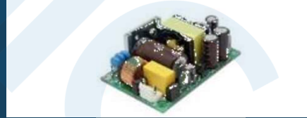
ASM65 AC-DC 2" x 3" Open Frame Enclosed and Dual Output Options 65W (Convection)
