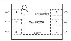
\* not connected: the pin can be freely left floating, or connected to GND, or connected to VCC
