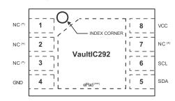
\* not connected => the pin can be freely left floating, or connected to GND, or connected to VCC \*\* the exposed pad is internally connected to GND. It is recommended (but not mandatory) to connect it to the board GND
